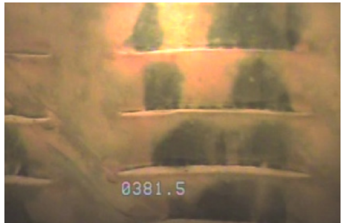
Figure 2. Louvered well screen covered with slime within days of being installed in new water well. Photo by G. Hix, 2012.
